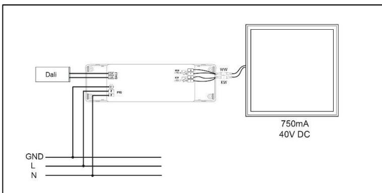
**B. Connection to any desired 750mA constant current LED driver**
